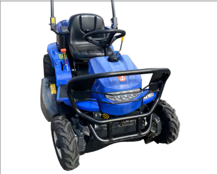
SRA950FA 21hp 95cm width deck Slope capability 25° 4WD
